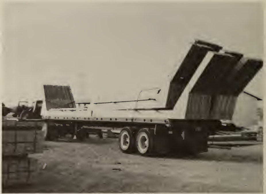
Truck load of Rigid Frame Rafters.
